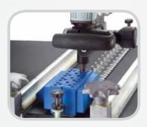
Increase operator efficiency with electric powered installation of BR6 fasteners.
