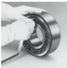
Fig. 1: Checking bearing clearance with bearing on bench.
